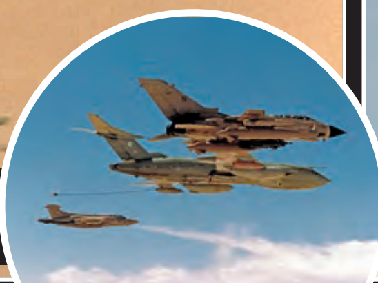
SUPPORT: A 55 Sqn Victor refuels a Tornado GR.1 and Buccaneer S.2 on their way to a target
