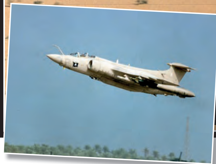
RAID: A 208 Sqn Buccaneer taking off from Muharraq, Bahrain, carrying a Paveway laser-guided bomb and Paveway targeting pod on the port wing weapons pylons
